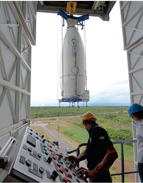
A mock payload segment for the new Vega launch vehicle is hoisted into position at Europe’s spaceport in French Guiana. A full-scale mock-up was assembled in February 2011 as part of testing procedures prior to the maiden launch planned for later in the year. Credit: ESA
