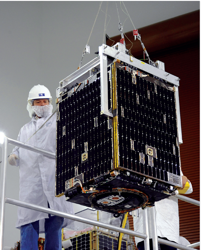
Technicians lift the STPSat-2 satellite to place it in the payload area of a Minotaur IV launch vehicle at Kodiak Launch Complex. The satellite was one of seven launched as part of the Space Test Program-S26 mission. The U.S. Department of Defense uses the Space Test Program to test experimental technologies that will enhance military operational capability. Credit: Jose (Lou) Hernandez
