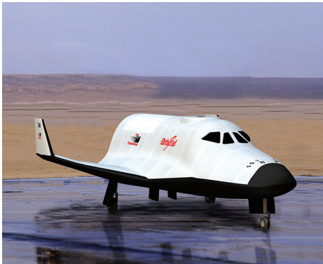
The spacecraft proposed by Orbital Sciences for NASA's CCDev 2 program would seat four astronauts and launch atop an expendable launch vehicle, such as the Atlas V rocket. The vehicle would return to Earth with a conventional runway landing. Credit: Orbital Sciences
