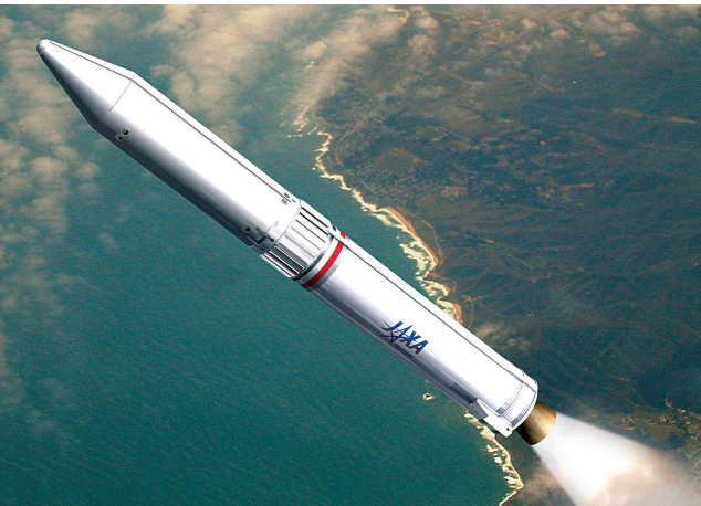
JAXA hopes to simplify and standardize the launch process, resulting in lowered costs and more frequent missions with the new Epsilon Launch Vehicle it is developing. In its standard configuration, Epsilon will lift 1,200 kilograms (2,650 pounds) into low Earth orbit. Credit: JAXA
