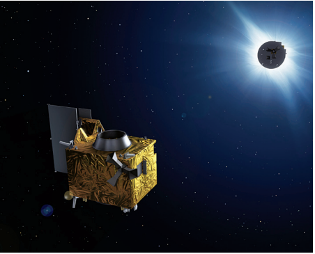
The two PROBA-3 spacecraft will test algorithms, sensors, propulsion systems, and other technologies needed for groups of small satellites flying in formation. One of the spacecraft will fly in such a way that it eclipses the Sun, allowing the second spacecraft to observe the solar corona. Credit: ESA/S. Corvaja
