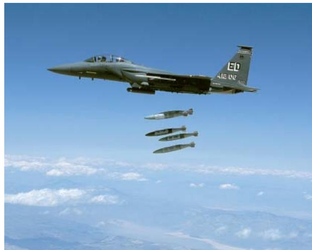
An F-15 Eagle is seen dropping MK-84 JDAMs. Each bomb can be individually targeted, which allows heavy bombers like the B-2 Spirit to drop 80 bombs at once and hit 80 pre-specified targets. Image credit: Edwards Air Force Base/ Bobbi Garcia
