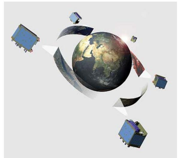
The RapidEye constellation will consist of five microsatellites capable of observing the entire world in high resolution every 24 hours. *Image credit: RapidEye AG*
