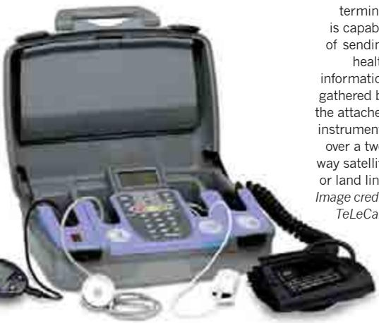
The TeLeCare terminal is capable of sending health information gathered by the attached instruments over a two-way satellite or land line. *Image credit: TeLeCare*
