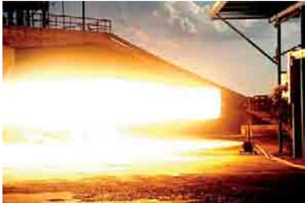
Based on a long heritage of space proven engines, Merlin is the highest performance gas generator cycle kerosene engine ever built. Nine Merlin engines will power the first stage of SpaceX's Falcon 9 rocket.
