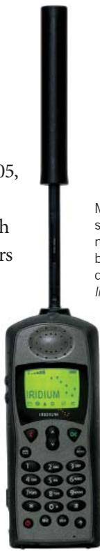
Mobile telephony services can provide near-global coverage by communicating directly with a satellite.
