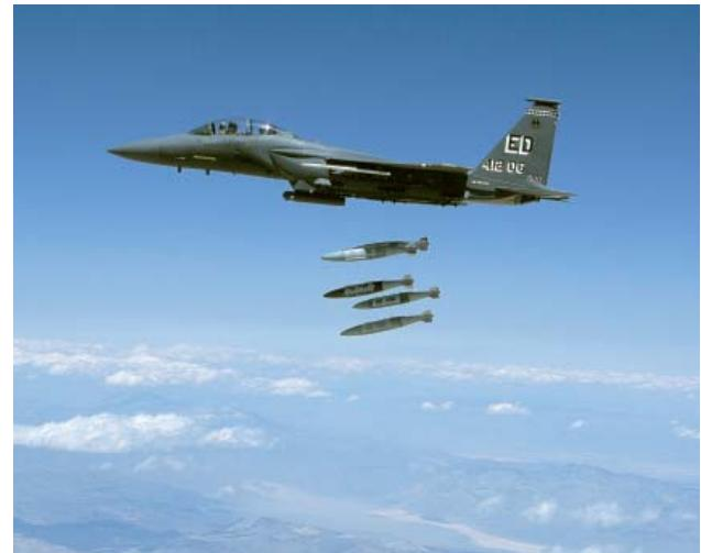
An F-15 Eagle is seen dropping MK-84 JDAMs. Each bomb can be individually targeted, which allows heavy bombers like the B-2 Spirit to drop 80 bombs at once and hit 80 pre-specified targets.
