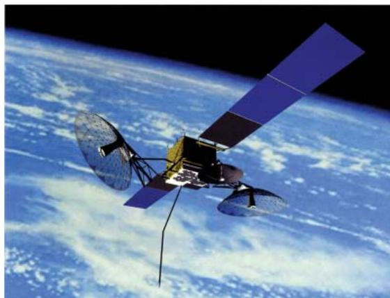
This high altitude satellite, part of the Tracking and Data Relay Satellite System (TDRSS) constellation, can maintain near continuous contact with lower orbiting satellites, replacing many of the ground stations once needed for communicating with satellites.
