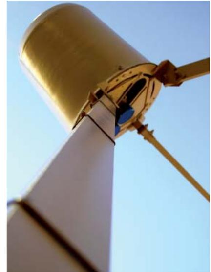
In this abstract view of a satellite feedhorn, we are peering down the brace. The feedhorn selects the polarity of the waves to be received, which helps to attenuate unwanted signals from adjacent channels and transponders, and from other communications satellites at nearby orbital positions. On a satellite dish, the feedhorn is what is mounted at the end of a mast from the center of the dish, or on tripod legs mounted to the edge of the dish.
