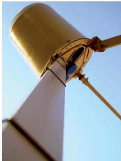
In this abstract view of a satellite feedhorn, we are peering down the brace. The feedhorn selects the polarity of the waves to be received, which helps to attenuate unwanted signals from adjacent channels and transponders, and from other communications satellites at nearby orbital positions. On a satellite dish, the feedhorn is what is mounted at the end of a mast from the center of the dish, or on tripod legs mounted to the edge of the dish.
