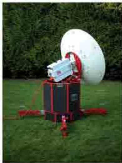
VSAT dish in remote setting readyed for transmissions. *Image credit: TC Communications*
