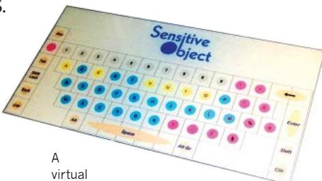
A virtual keyboard that can be applied to a variety of materials is being developed with technology previously used on accelerometers in the inertial positioning system onboard Ariane launches. Vibration sensors are mounted on the product to detect which area is touched. It is easy to maintain and has no moving parts. *Image credit: Sensitive Object*
