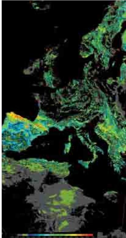
Realtime Normalized Difference Vegetation Index (NDVI) data from a NOAA Advanced Very High Resolution Radiometer (AVHRR). NDVI is a quantity that measures greenness and vigor of vegetation. Image credit: RSGB, University of Bern, and NOAA
