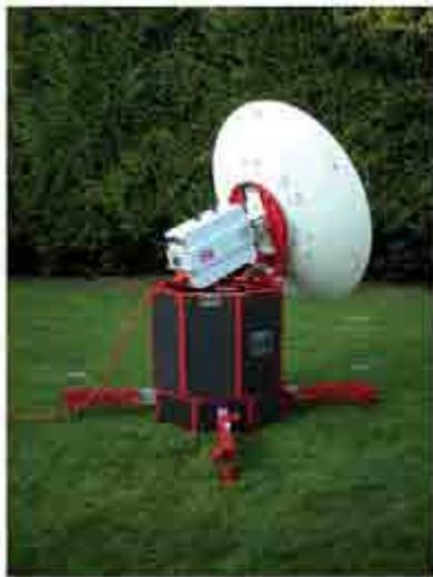
VSAT dish in remote setting readied for transmissions. Image credit: TC Communications
