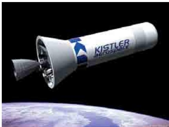
Rocketplane's K-1, one of two recipients of COTS funding, is a fully reusable aerospace vehicle designed to accommodate a wide range of missions including LEO payload delivery, microgravity missions, and reboost services for the ISS.
