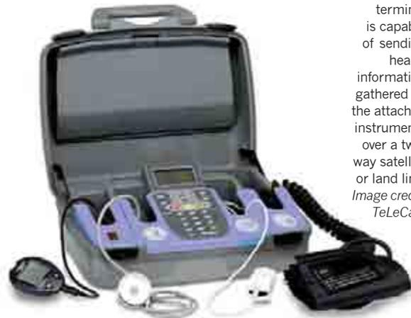
The TeLeCare terminal is capable of sending health information gathered by the attached instruments over a two-way satellite or land line. Image credit: TeLeCare
