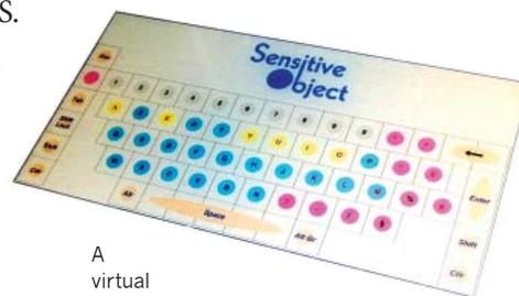
A virtual keyboard that can be applied to a variety of materials is being developed with technology previously used on accelerometers in the inertial positioning system onboard Ariane launches. Vibration sensors are mounted on the product to detect which area is touched. It is easy to maintain and has no moving parts. Image credit: Sensitive Object
