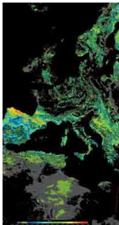
Realtime Normalized Difference Vegetation Index (NDVI) data from a NOAA Advanced Very High Resolution Radiometer (AVHRR). NDVI is a quantity that measures greenness and vigor of vegetation.
