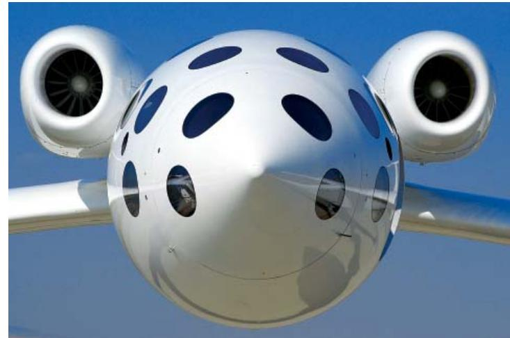
The White Knight is a manned twin-turbojet aircraft designed to provide a high-altitude airborne launch of SpaceShipOne. *Image credit: Scaled Composites*
