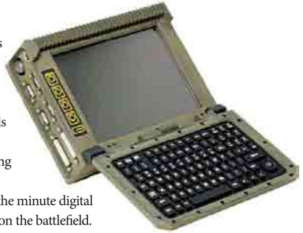
DRS's Handheld Terminal Unit (HTU) provides the soldier a small, lightweight, rugged, fully-sealed computing device. Highlighted by GPS and TCIM (Tactical Communications Interface Modem), the HTU is based solely on commercial off-the-shelf technology. *Image credit: DRS Technologies, Inc.*
