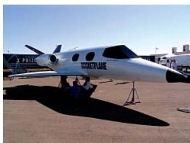
Powered by two jet engines and a rocket engine, the Rocketplane XP is a heavily modified Learjet 25 capable of reaching sub-orbital space.
