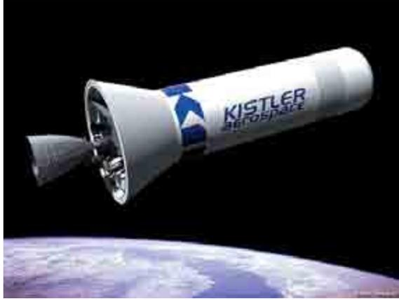
Rocketplane's K-1, one of two recipients of COTS funding, is a fully reusable aerospace vehicle designed to accommodate a wide range of missions including LEO payload delivery, microgravity missions, and reboost services for the ISS. *Image credit: Rocketplane Limited, Inc.*
